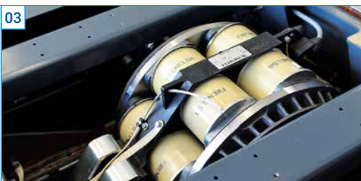
Eddy-current brake for performance measurement and load simulation: maximum 7000 N tractive force per brake, 14,000 N per axle with two brakes, maximum expansion level is four brakes on the 4WD dynamometer. Boost function including temperature monitoring on the brakes, especially for performance measurement on electric vehicles.
