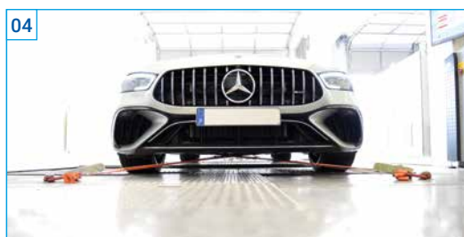
Professional vehicle fixing for the highest safety levels, as well as reproducibility of measurements.
