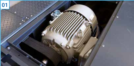
E-motor for all-wheel synchronisation: tracking acceleration on the non-driven axle MSR 3000: 1.5 m/s 2 up to 200 km/h (30 kW) MSR 3000: 1.0 m/s 2 up to 240 km/h (30 kW) MSR 5000: 3.0 m/s 2 up to 300 km/h (37 kW)
